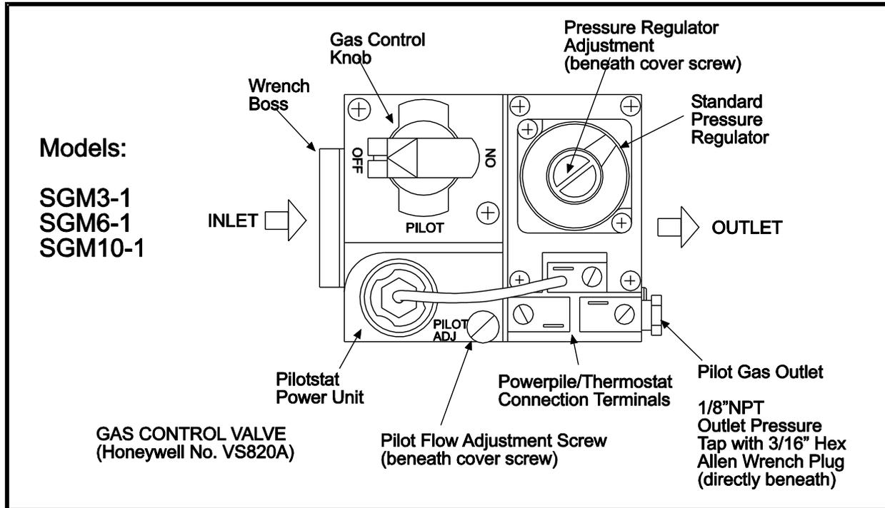
2. With the main burner operating, check the burner manifold pressure using a water manometer. Gauges that measure pressure in pounds per square inch are not accurate enough to measure or set the manifold pressure. All measurements **MUST BE** made when this heater and all other gas burning equipment that is connected to the gas supply system are operating at maximum capacity.
