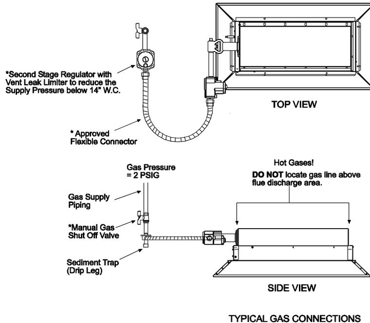
5. This appliance is equipped with a snap-opening, combination gas valve. The maximum supply pressure to the appliance is 14" W.C. or 1/2 P.S.I. If the line pressure is more than the maximum supply pressure, then use a line regulator as indicated in the following illustration, or a line regulator which corresponds to the supply pressure.
